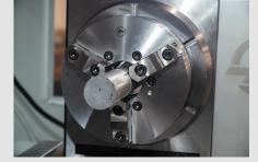
Our featured product this month is the selfcentering 3-jaw chuck—a shop staple known for its fast setup and dependable hold. Ideal for cylindrical workpieces, it reduces setup time and ensures concentricity with every use. Find out why it's the go-to solution for turning shops worldwide
